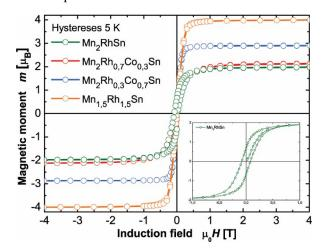
Fig. 3: Magnetic properties of  $Mn_{2-x}Rh_{1+x}Sn$  and  $Mn_2Rh_{1-x}Co_xSn$ . The MH-curves were measured at T = 5 K. The inset shows the zoomed-in view of the hysteresis curves at T = 5 K for  $Mn_2RhSn$ .
