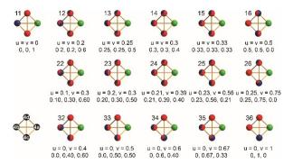
Fig. 1: Different types of substitutional disorder (X,Y)for the cubic Heusler structure of composition  $X_2YZ$ . The Z component fully occupies Wyckoff position 4a. For each type of disorder, the bcc tetrahedron is shown. The general formula is  $(X_{1-w}Y_u)^{4d}(X_{1-w},Y_v)^{4c}(X_{u+v},Y_{1-u-v})^{4b}Z^{4a}$ . Parameters in second row at the bottom of each bcc tetrahedron are occupancy factors of Y for 4d, 4c, and 4b sites in F-43m.
