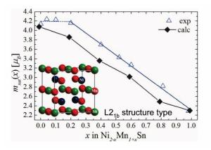
Fig. 2: The saturation magnetization  $m_{sat.}$  at 1.8 K. from magnetometry and theoretically calculated as a function of the Mn content. The inset shows the inverse Heusler structure of Mn<sub>2</sub>NiSn, which becomes the L2<sub>1b</sub> structure type in case of random mix occupation of the heterocubic sites by (Ni,Mn).
