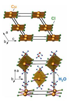
FIG. 5. (Color online) Sketch of the magnetically active  $pd\sigma$  plaquette for CuCl<sub>2</sub> (top) and CuCl<sub>2</sub>·2H<sub>2</sub>O (bottom). Whereas these orbitals form quasi-1D edge-shared chains in CuCl<sub>2</sub>, the plaquettes in CuCl<sub>2</sub>·2H<sub>2</sub>O are isolated, resulting in weak but 3D interactions.
