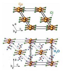
FIG. 1. (Color online) Crystal structures of  $CuCl_2$  (top) and  $CuCl_2 \cdot 2H_2O$  (bottom). The shortest Cu-Cl bonds are highlighted (brown). The crystal water is intercalated between the  $CuCl_2$  layers. The dashed line in the  $CuCl_2 \cdot 2H_2O$  structure marks the unit cell of the water-free  $CuCl_2$ .
