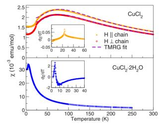
FIG. 2. (Color online) Magnetic susceptibility of single crystalline CuCl<sub>2</sub> (top) and CuCl<sub>2</sub>·2H<sub>2</sub>O powder (bottom) as a function of temperature ( $\mu_0H=1$  T). TMRG fits are given by the dashed lines. The insets show the derivative  $d\chi/dT$ ; the ordering temperatures are indicated by sharp peaks.
