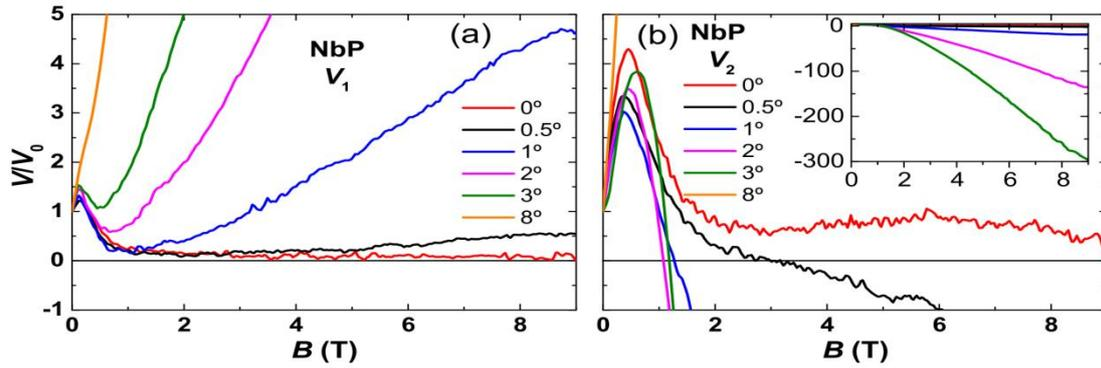
Fig.-6: (a) and (b) magnetic field dependence of the voltage for different angles  $\theta$  between the magnetic field and the electrical current for the two contact pairs  $V_1$  and  $V_2$ , respectively. The inset in (b) displays the region where a negative voltage is observed for the contact pair  $V_2$  (taken from Ref. 9).
