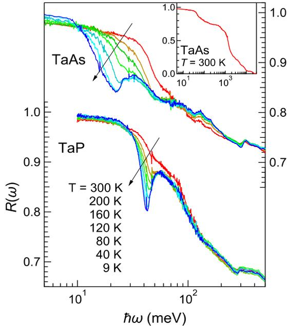
Fig.-3: Temperature-dependent reflectivity  $[R(\omega)]$  spectra of TaP and TaAs in the photon-energy region of 5–500 meV. The two compounds both show a Drude behavior at the lowest-energies with clearly different pronounced temperature dependence. The inset shows the  $R(\omega)$  spectrum of TaAs at 300 K in the whole measured region up to 30 eV [3].
