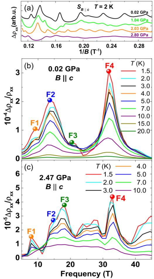
Fig.-5: (a) Shubnikov–de Haas oscillations as a function of the inverse magnetic field taken at different pressures for  $B||c$ . (b) and (c) Temperature dependence of the fast Fourier transform of the SdH oscillations (taken from Ref. 7).
