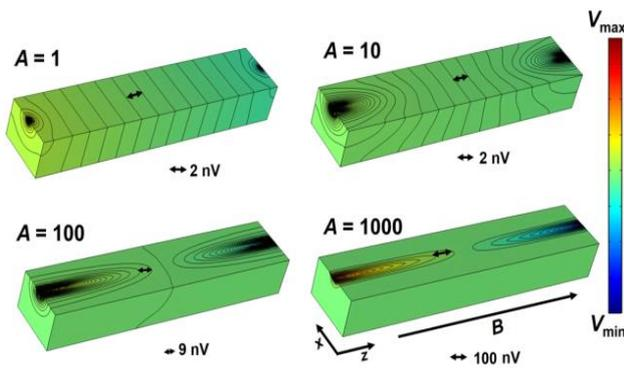
Fig.-7: Calculated potential distribution for different resistance anisotropies  $A = \rho_{xy}/\rho_{zz} = 1, 10, 100,$  and  $1000$  for a sample with point-like current electrodes. The current contacts are in the middle of the upper edge of the face sides.  $B$  is aligned with the current electrodes,  $\rho_{zz}$  ( $\rho_{xx}$ ) is the resistance parallel (perpendicular) to  $B$ . The lines are contour lines of the equipotential surfaces (taken from Ref. 9).
