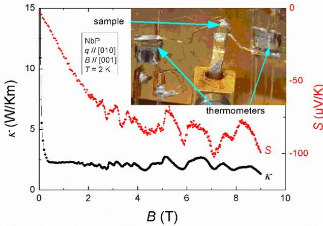
Fig.-4: Field dependence of the adiabatic thermopower (right scale) and the thermal conductivity (left scale) in NbP single crystal [8].
