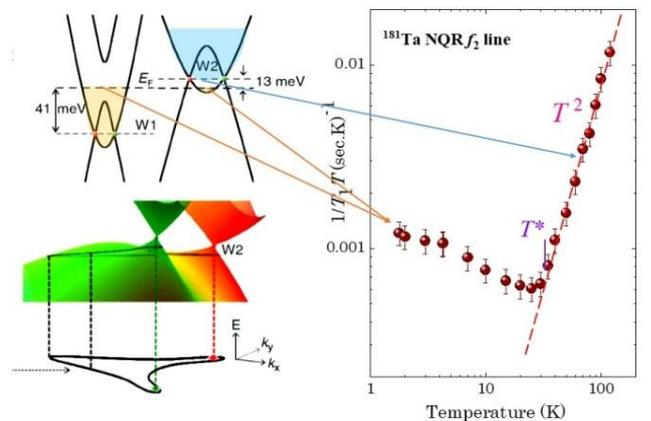
Fig.-2: (right)  $T$ -dependence of  $1/T_1 T$  obtained from Ta NQR in TaP. Above  $T^* \sim 30$  K characteristic Weyl fermion excitations from the W2 points (dashed line) with  $1/T_1 T \propto T^2$  behavior could be observed. For  $T < T^*$  the Korringa relaxation with a temperature dependent chemical potential is valid [2].
