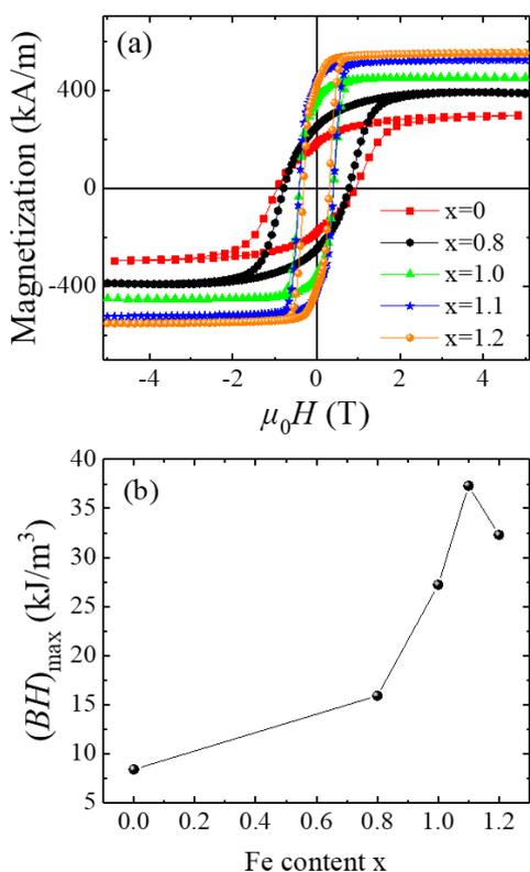
Fig.-4: (a) Typical out-of-plane magnetization curves and (b)  $(BH)_{\max}$  values of  $\text{Mn}_{2.7-x}\text{Fe}_x\text{Ga}_{1.3}$  films with different Fe contents  $x$ .
