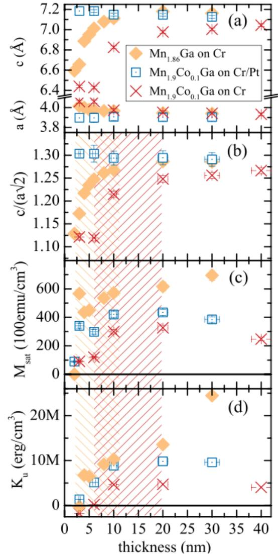
Fig.-2: (a) Lattice constants, (b) tetragonality, (c) saturation magnetization, and (d) effective anisotropy of the different Mn-Ga films.
