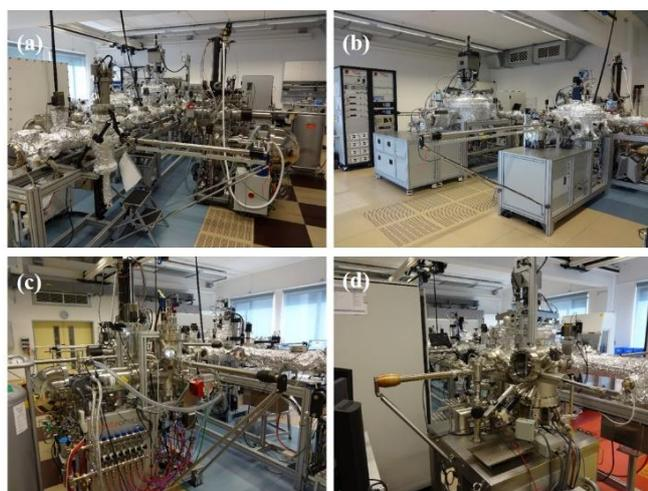
Fig.-1: (a) State-of-the-art UHV cluster tool for the growth and characterization of thin films. (b) Two sputter deposition systems, (c) the MBE and ARPES systems and (d) the UHV scanning probe microscope.
