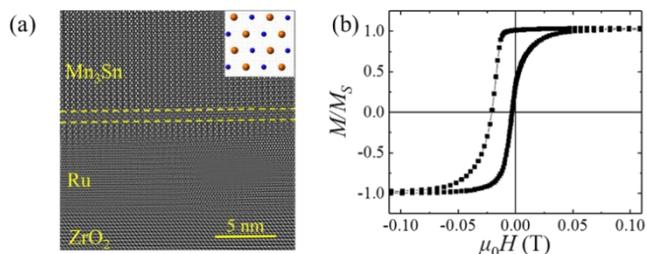
Fig.-6: (a) Cross-section HRTEM image of  $\text{Mn}_3\text{Sn}$  film and (b) in-plane magnetization hysteresis loops of the  $\text{Mn}_3\text{Sn}(40 \text{ nm})/\text{Py}(5 \text{ nm})$  bilayer at 5 K after I-T field cooling.
