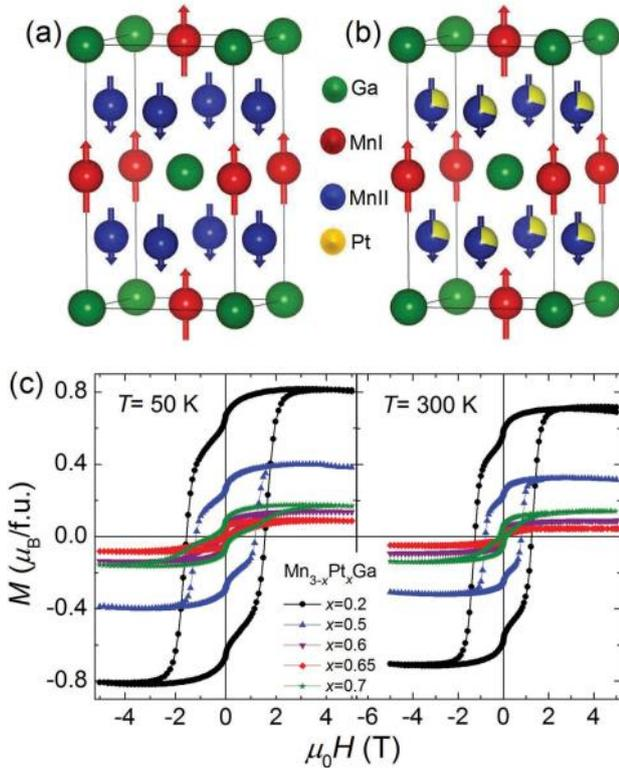
Fig.-3: (a) Crystal and magnetic structure of  $\text{Mn}_3\text{Ga}$ . (b) Crystal and magnetic structure of  $\text{Mn}_{2.4}\text{Pt}_{0.6}\text{Ga}$ . (c) Out-of-plane magnetization hysteresis curves of  $\text{Mn}_{3-x}\text{Pt}_x\text{Ga}$  thin films measured at 50 K and 300 K.
