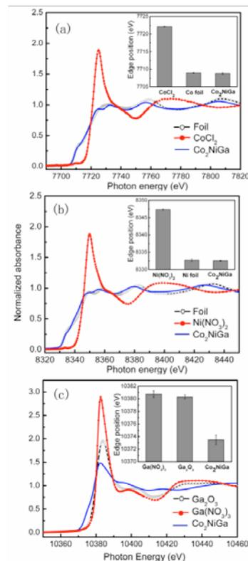
Fig. 3: XANES data for the  $\gamma\text{-Co}_2\text{NiGa}$  nanoparticles at the absorption edges of Co (a), Ni (b), and Ga (c).
