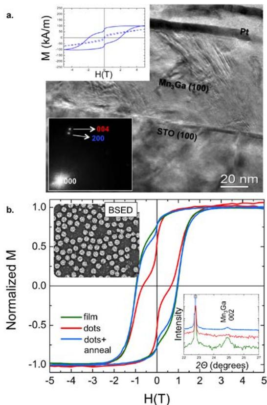
Fig. 2: (a) Cross sectional HRTEM image from the  $x=0.75$ ,  $350^\circ\text{C}$  sample. The bottom inset shows a portion of the FFT in the film region. The top inset shows in-plane (dashed) and out-of-plane (solid) magnetization. (b)  $M(H)$  for  $\text{Mn}_{70}\text{Ga}_{30}$  film and nanodots before and after annealing. The bottom inset shows an XRD pattern of the same samples. The top inset shows an SEM image of the nanodots.
