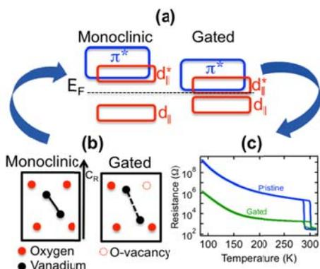
**Fig 3.** Interconnection between crystal and electronic structure of monoclinic and gated  $\text{VO}_2$ . (a) Modifications in the band diagram can be described by a reduction of  $d_{||}$  band splitting (b) Structural changes induced by electrolyte gating: in the gated structure, the V-V distances are larger than that in the monoclinic phase (c) Temperature-dependent resistances of pristine and gated films.
