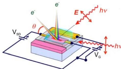
**Fig.1.** Experiment and device schematic. The Au gate electrode and electrical contacts are shown in yellow. The oxide film is shown in pink and is set at a distance 0.5 mm from the gate. The turquoise droplet is the ionic liquid.
