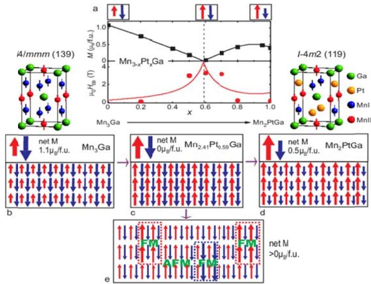
FIG 2. Design of a compensated magnetic state in  $\text{Mn}_{3-x}\text{Pt}_x\text{Ga}$ . Perfect magnetic compensation is expected in  $\text{Mn}_{2.41}\text{Pt}_{0.59}\text{Ga}$  by changing the composition from  $\text{Mn}_3\text{Ga}$  to  $\text{Mn}_2\text{PtGa}$ . FM domains appears inside the compensated AFM host due to antisite disorder in the sample .
