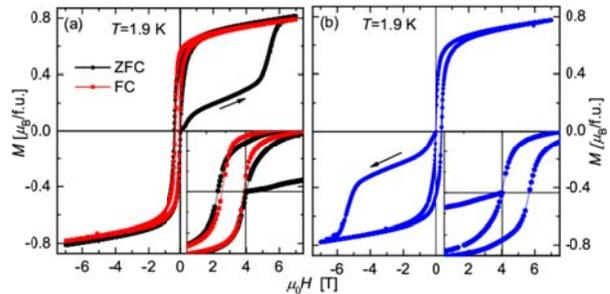
FIG. 1. (a) Zero field cooled (ZFC) and field cooled (FC)  $M(H)$  loops for  $Mn_2PtGa$  measured at 1.9 K. The measurements are performed as  $0 \rightarrow +7$  T  $\rightarrow -7$  T  $\rightarrow +7$  T (b) ZFC  $M(H)$  loop at 1.9 K performed as  $0 \rightarrow +7$  T  $\rightarrow -7$  T  $\rightarrow +7$  T. The insets show a magnified view of  $M(H)$  loops around  $H = 0$ .
