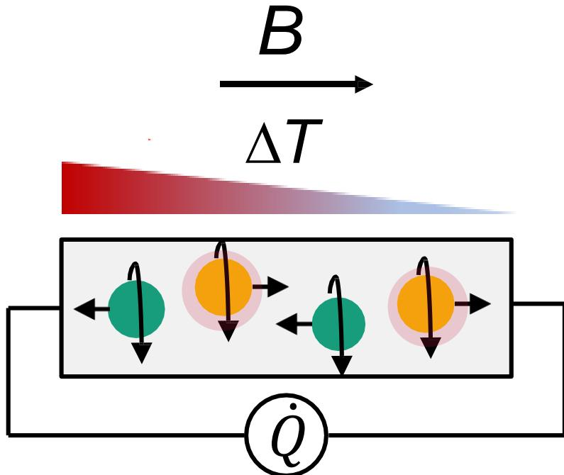
$$K_{\text{th}} = \dot{Q} / \Delta T = d_{\text{th}} + c_2 a_g B_{\parallel}^2$$
