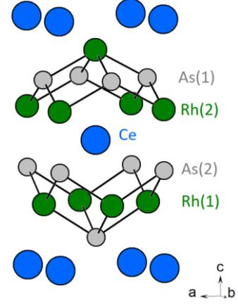
Fig. 4: Crystal structure of  $\text{CeRh}_2\text{As}_2$ .
