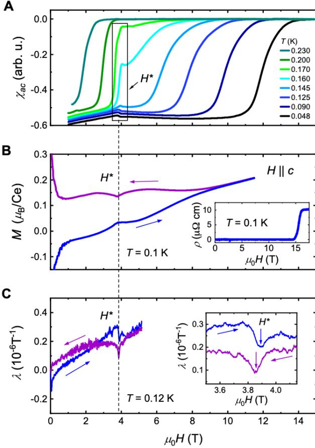
Fig. 2: Magnetic field dependence of the ac-susceptibility (A), the magnetization (B) and the magnetostriction (C) for  $H \parallel c$ . The inset in (B) shows the resistivity and the inset in (C) zooms in on the data in (C) around the kink.
