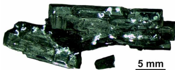
Fig. 3: Crystals of \text{K}_2\text{Te}_3 obtained from hydroflux.
