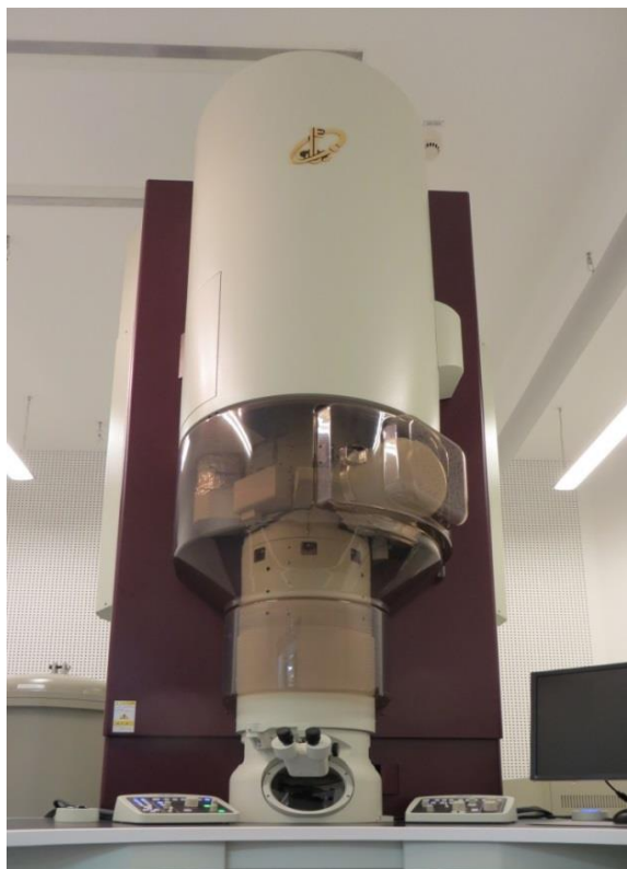
Fig.-1: The Dresden Grand ARM, the JEM-ARM300F with double C_s -correction by JEOL – nick-named the "Grand ARM" – in its custom-built booth.
