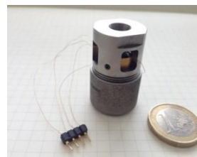
Fig.-1: Custom-designed miniature diamond anvil cell used for studies of structural, optical, magnetic, and electronic properties of materials at pressures up to 100 GPa.
